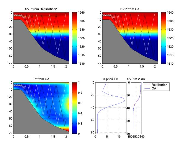
Figure 15: Yoyo control implementation. Afternoon 7/19/05. sound\_faf05\_jul19\_01\_day0\_0.5\_sec1.mat. Black line is the forward path; White line is the backward path; Red star is the sound source location; Green line is receivers' location. Note that to avoid bottom AUV turns around at 5 m above bottom.
