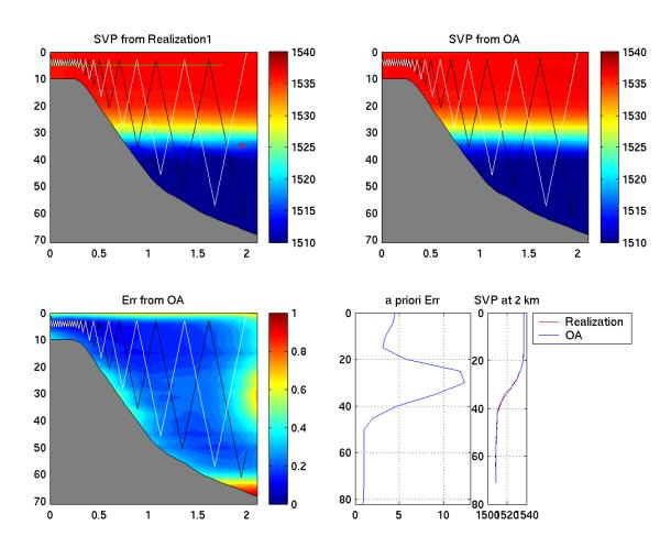
Figure 13: Yoyo control implementation. Morning 7/19/05. sound\_faf05\_jul19\_01\_day0\_0.5\_sec1.mat. Black line is the forward path; White line is the backward path; Red star is the sound source location; Green line is receivers' location. Note that to avoid bottom AUV turns around at 5 m above bottom.
