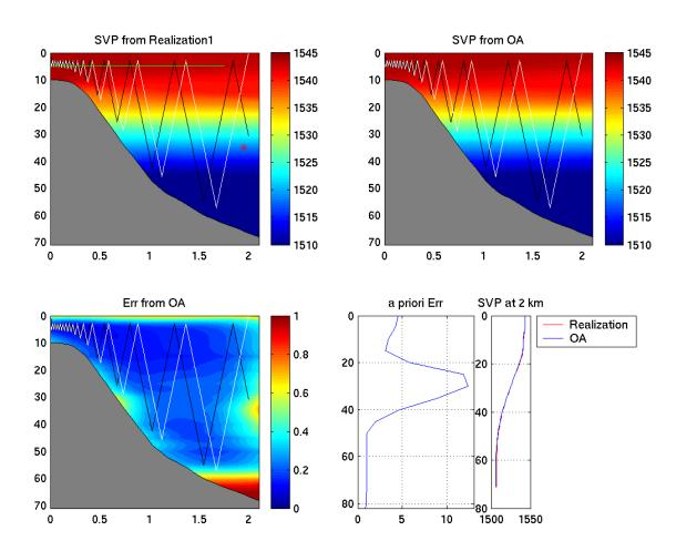
Figure 31: Yoyo control implementation. Morning 7/23/05. sound\_faf05\_jul22\_14\_day1\_2\_sec1.mat. Black line is the forward path; White line is the backward path; Red star is the sound source location; Green line is receivers' location. Note that to avoid bottom AUV turns around at 5 m above bottom.
