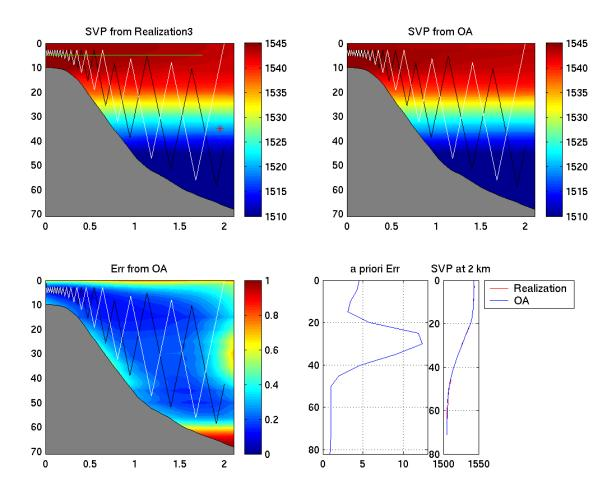
Figure 35: Yoyo control implementation. Morning 7/24/05. sound\_faf05\_jul22\_14\_day1\_2\_sec1.mat. Black line is the forward path; White line is the backward path; Red star is the sound source location; Green line is receivers' location. Note that to avoid bottom AUV turns around at 5 m above bottom.
