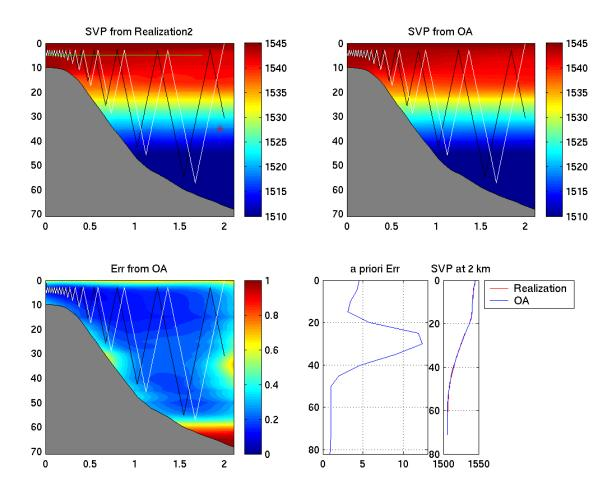
Figure 33: Yoyo control implementation. Afternoon 7/23/05. sound\_faf05\_jul22\_14\_day1\_2\_sec1.mat. Black line is the forward path; White line is the backward path; Red star is the sound source location; Green line is receivers' location. Note that to avoid bottom AUV turns around at 5 m above bottom.
