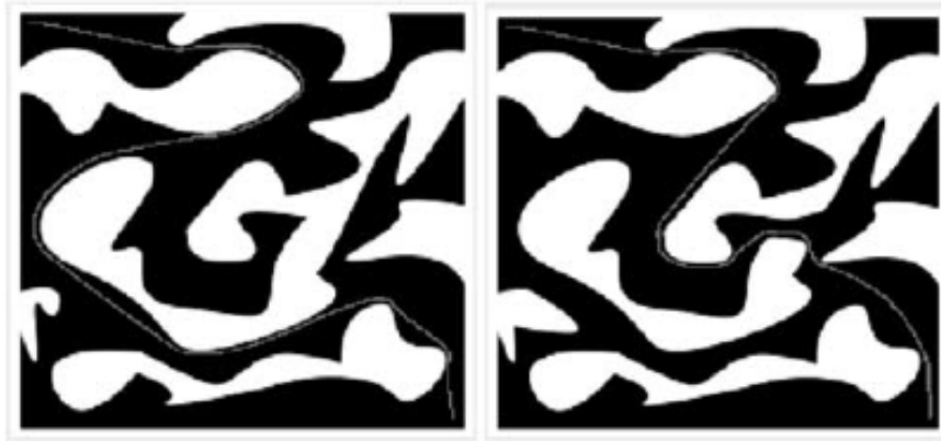
Figure 2-6: Path planning with lifelong Fast Marching Method (reprinted from (Evans et al., 2008))
